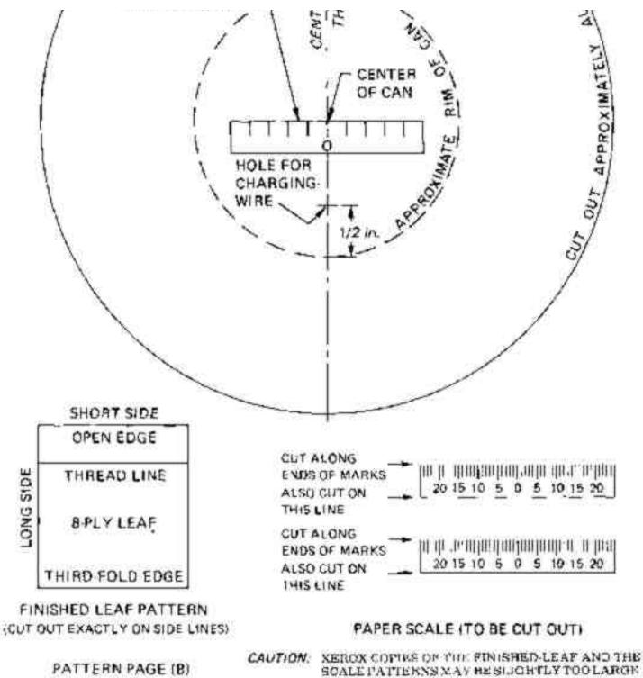
7. While holding a straight edge along the THREAD LINE of the pattern, press with a sharp pencil so as to make a shallow groove for the THREAD LINE on the 8-ply aluminum sheet. Also using a sharp pencil, trace around the top and side of the pattern, so as to indent (groove) the 8-ply foil.
