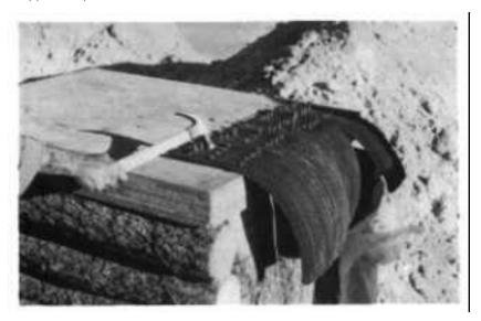
**Fig. D.16. Blast-tested triangular blast door made of hand-hewn pine poles, notched and nailed together.** This door closed on a triangular pole base that is concealed in this photo by two of the three blast-protector logs that also withstood 53-psi blast effects.
