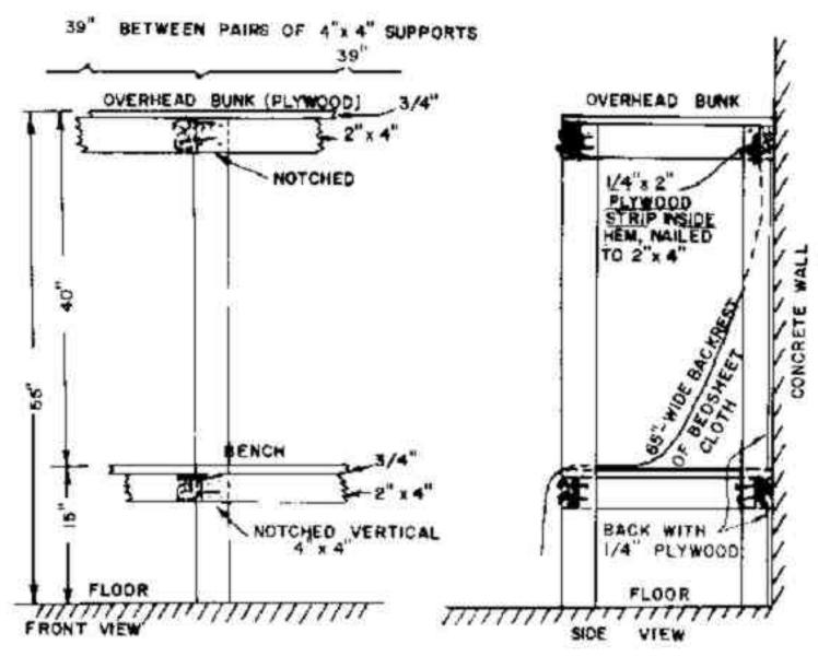
Fig. 17.5. Backrests of Bedsheet Cloth and 2-Inch-Thick Pads Make Sitting and Sleeping Comfortable.
