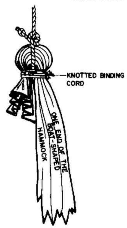
10. Repeat the procedure (4 through 9) with the other end of the double-folded sheet, thus producing a boat-shaped hammock with its two sides each about 8 inches shorter than its lengthwise center section.
