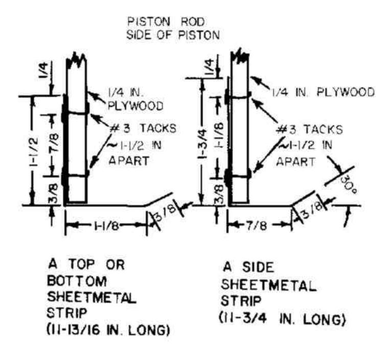
g. With the sheetmetal strip held sandwiched between the two 12-1/4-in.-long boards by the two "C" clamps and the vise, so that the bending line for the almost 90-degree bend is barely visible, bend the exposed part of the strip 90 degrees, in the same direction that the 3/8-in.-wide part was bent. See Figs. 13 and 14.
