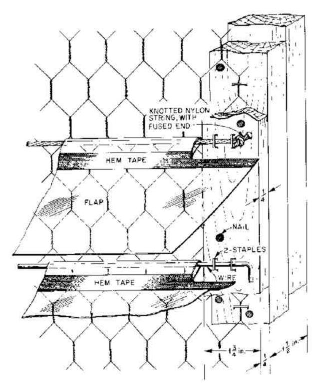
Note in Fig. 13 that each pivot-wire is held firm and straight by 2 staples securing each end. The wire used should be at least as springy as coat hanger wire. If string is used instead of wire, nylon cord about the diameter of coat hanger wire is best for the pivot-strings.
