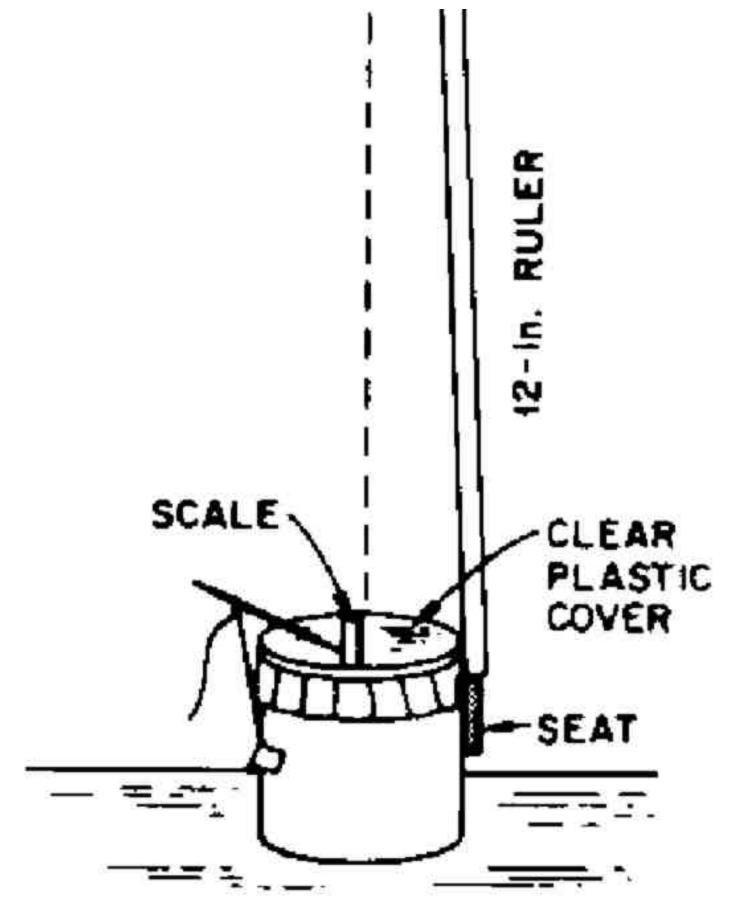
To read the separation of the **lower** edges of the two KFM leaves with one eye, look straight down on the leaves and the scale on the clear plastic cover. Keep the reading eye 12 inches above the SEAT. The KFM should be resting on a horizontal surface. To be sure the reading eye is always at this exact distance, place
