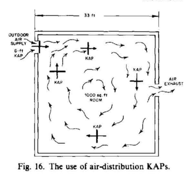
You should make and use enough KAPs to cause air movement that can be felt in all parts of your shelter. Remember that if KAPs are installed near the floor and the shelter is fully occupied, the occupants' bodies will partially block the pumped airflow more than if the same KAPs were suspended overhead.
