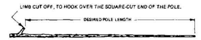
(5) It usually is best first to cut the poles exactly two or three times the final length of the poles to be used in the shelter.
