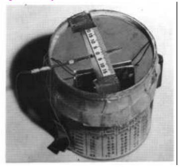
B. Charging a KFM by a Spark-Gap Discharge from a Tape That Has Been Electrostatically Charged by Being Unwound Quickly. Note that the charged tape is moved so that its surface is perpendicular to the charging-wire.
