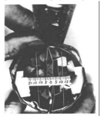
C. A Charged KFM. Note the separation of the upper edges of its two leaves. The chargingwire has been raised to an almost horizontal position so that its lower end is too far above the aluminum leaves to permit electrical leakage from the leaves back up the charging-wire and into the outside air.
