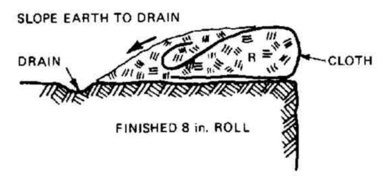
(6) If a greater thickness of rolls is needed, level the earth on top of a roll; then make another earth-filled roll on this level surface.
