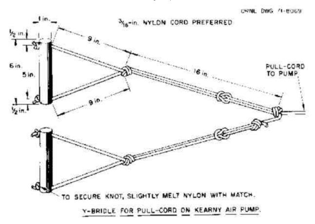
A man of average size and strength can operate a 6 ft X 29 in. KAP by himself, pumping over 4000 cubic feet per minute through a typical large shelter without working hard; tests have shown that he must deliver only about 1/20 of a horsepower. However, most people prefer to work in pairs when pulling a 6-ft KAP equipped with a "Y" bridle, when pumping over 3000 cfm.
