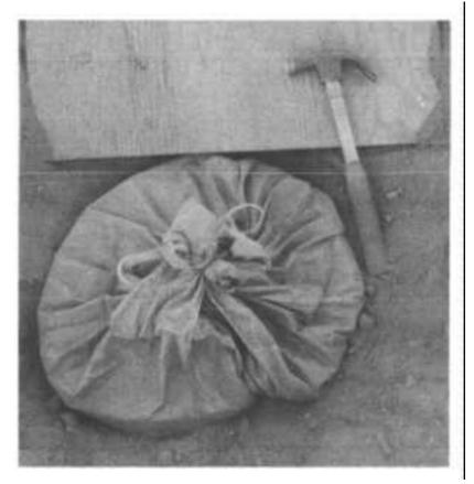
**Fig. 8.5. Post-blast view of plastic-lined water storage pit undamaged at a 6.7-psi overpressure range.** This pit held about 200 gallons.
