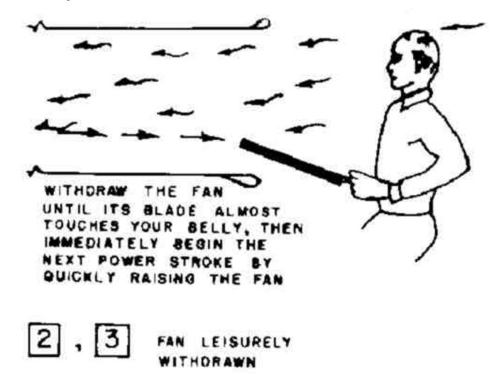
1) Quickly raise the fan to a vertical position close in front of your face and immediately fan (push) a slug of air into the opening - ending the power stroke with your arms fully extended and with the fan almost horizontal and out of the way of air that was "sucked" behind the fan and is still flowing out through the opening.
