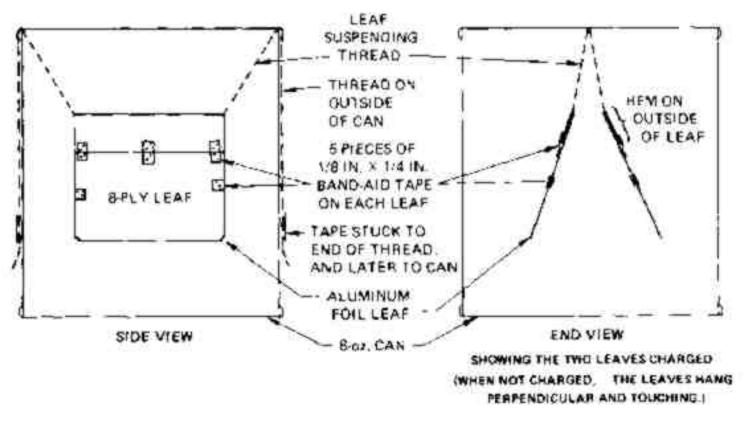
19. To prevent possible partial discharge from overly sharp lower corners of the leaves, use scissors to cut about 1/16 inch ( L) off each lower corner of the two leaves. (Partial discharge from an overly sharp corner may prevent a KFM's leaves from being adequately charged and adequately separated.)
