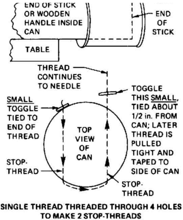
6. The stop-threads can be installed by using a needle to thread a single thread through all four holes. Use a very clean thread, preferably nylon, and do not touch the parts of this thread that will be inside the can and will serve as the insulating stop-threads. Soiled threads are poor insulators.
