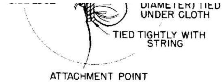
4. To make an attachment point for a chair "arm", hold a pebble (or a lump of earth) under one of these last marks, pull the double-thickness cloth tight around the pebble, and tie it in place. (See illustration.) Repeat on the other side-edge of the hammock.
